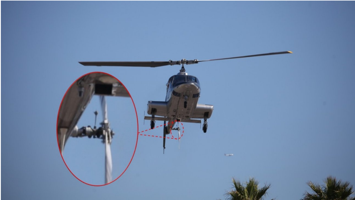
Figure 1. The accident helicopter before landing. A red callout shows a zoomed in view of the tail rotor assembly and a disconnected pitch link.
